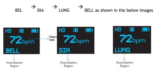
The BELL mode frequencies are from 50-200Hz. In this mode the user can hear low frequency sounds.
