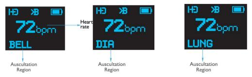
The BELL mode frequencies are from 50-200Hz. In this mode the user can hear low frequency sounds.
